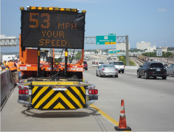
Signage w/ Radar
