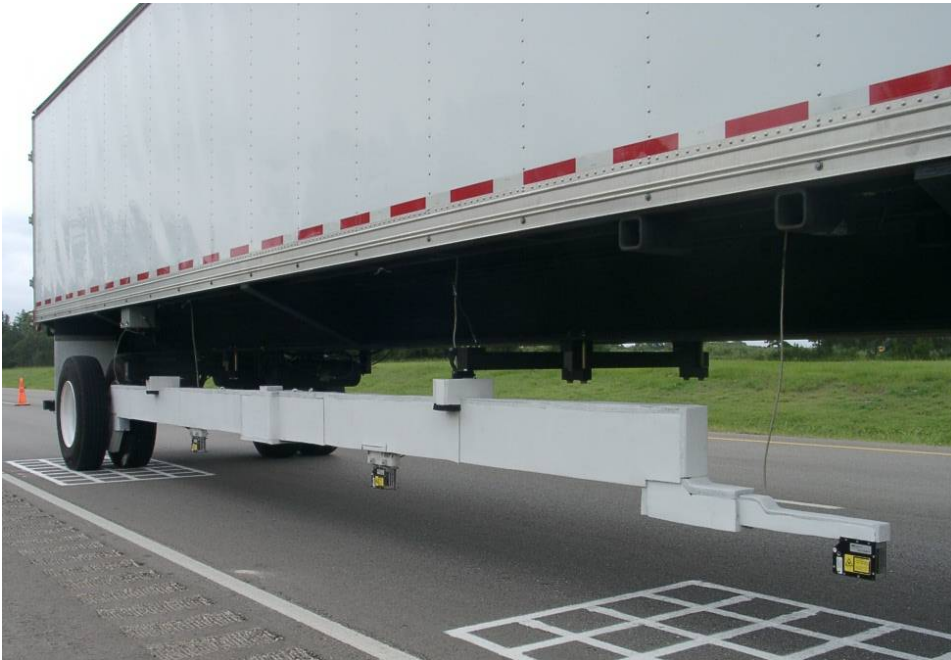
Reference beam and spot lasers
